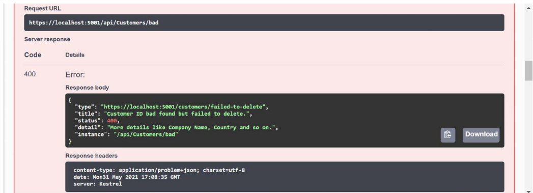
Figure 15.12: The customer did exist but failed to be deleted
